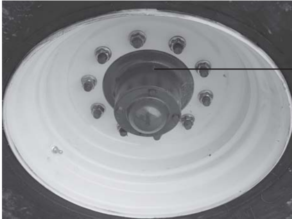
Wheel Hub Zerk (1 on each wheel hub)
